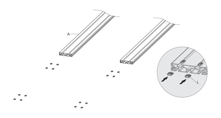
Note: Ensure the gap between the nuts halves on both sides are equal.
