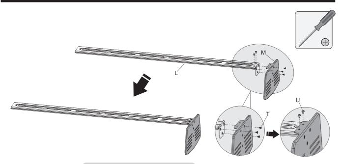
Attach the camera shelf to the connecting plate with the appropriate screws. Tighten all screws using a proper Phillips screwdriver.
