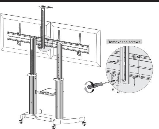
Attach the connecting plate to the universal plate with the removed screws. Tighten all screws using a proper Phillips screwdriver.
