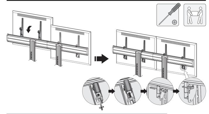
Hook the adapter brackets (attached the display) onto the universal plate.
