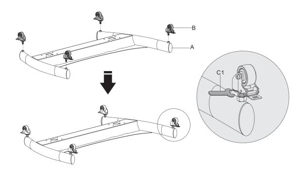
Note: Each caster can be adjusted independently for fine tuning. Slightly turn the nut to lower or raise the base.
