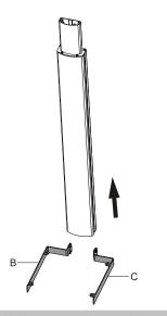
Slide the support arms along the column rails to the desired height.
