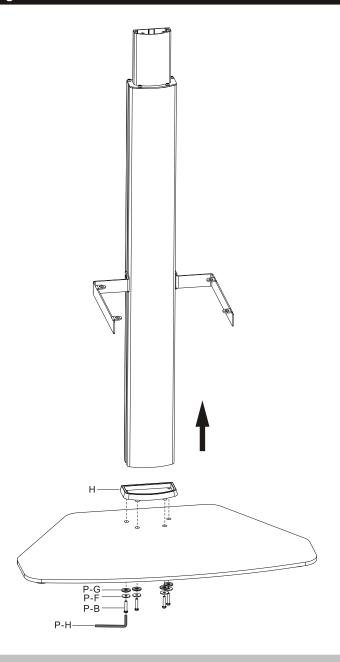
Attach the column and the foot pad to the base using the correct screws and washers. Tighten all screws with Allen key.
