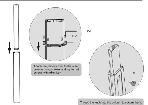
Insert the inner column into the outer column .
