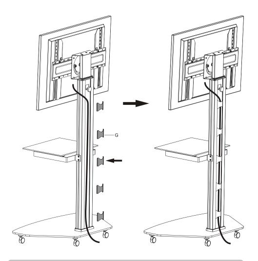
Route the cables along the column. Attach the cable cover to the column to hold the cables in place.
