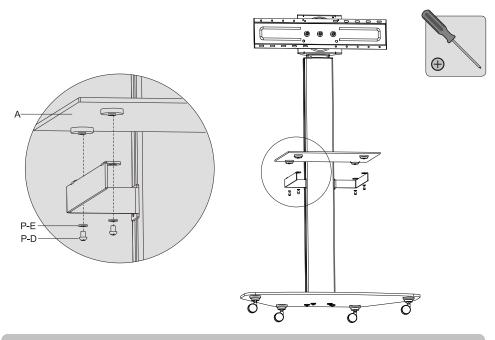
Attach the glass shelf to the installed support arms using the screws and washers, and tighten all screws with a proper screwdriver.
