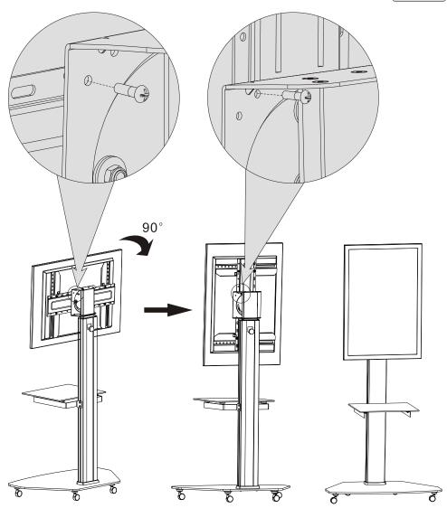
Remove the screw on the top plate to rotate the TV (with attached brackets and top plate at  $90^{\circ}$ ), Secure with just removed screw into a different position.
