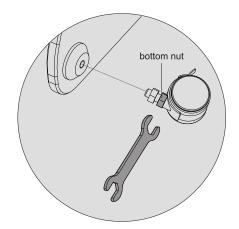
Install the casters into the base holes and tighten bottom nuts of the casters to the desired height.
