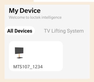
The home page consists of the product lists where you can view the added devices. Hold the device to edit i.e. delete or rename. Click the device to enter the device control page.
